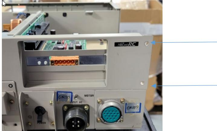
3. Remove empty PCI port cover by removing 1 screw, remove panel to allow installation of Ethernet card.
