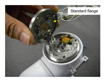
**Step 5**. Carefully attach the Electric Gripper Hand making sure the **Knock Pin** and the **Knock Pin Hole** are aligned.
