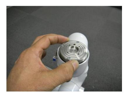
Step 3. Remove the (4) bolts that secure the Standard Flange.
