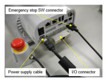
**Step 2.** Connect to the COBOTTA with your PC using the LAN cable. This PC needs to have Virtual TP installed.
