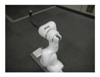
**Step 2.** Attach the Camera to the COBOTTA using the (2) M2.5X10 bolts, tightening torque is = 0.6Nm
