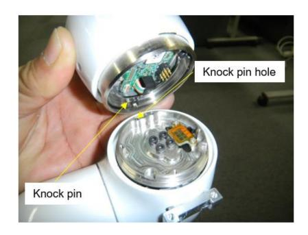
**Step 6.** Secure the Electric Gripper using the special spanner wrench (Part # 998997-1840) and rotating in the direction shown below. (Do not overtighten). Make sure that J6 is not against the mechanical + or – hard stop when you are tightening.
