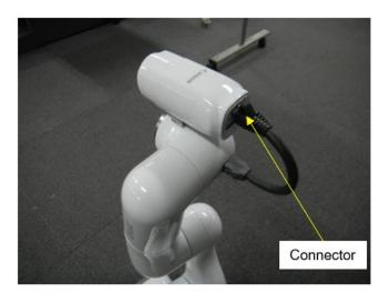
Step 3. Remove the (2) M3 bolts that secure the camera to the COBOTTA.
