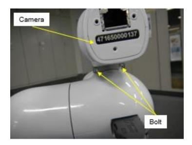
**Step 3**. Connect the cable from the Camera to the COBOTTA as pictured below.
